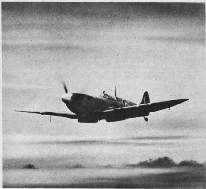
SPITFIRE IX Spitfires have elliptical wings with dihedral stemming from the roots. In head-on view wing radiators are clue to the IX.
